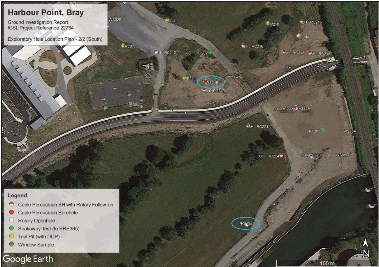
Figure 10-7 Perched Water & Groundwater Monitoring Well Location Map 2 of 2 (IGSL, 2021) (monitoring wells circled in blue)
