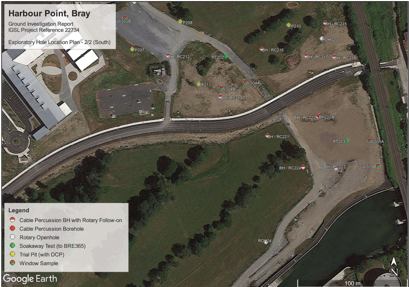
Figure 9-2 Ground Investigation Locations (including Environmental Sampling and Gas/Groundwater Monitoring Locations) Map 2 of 2 (IGSL, 2021).
